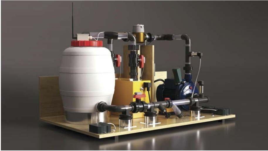
JOIN's Portable Living Lab can be used to simulate process phenomena such as cavitation.
